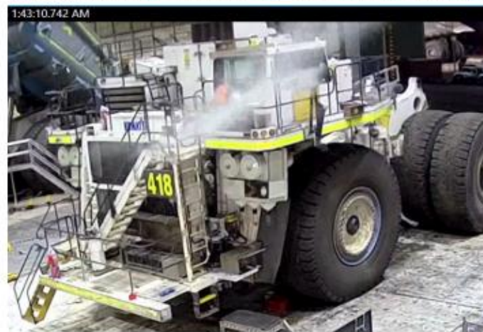
Figure 3: Release of uncontrolled energy - brake system hose whipping about releasing oil
