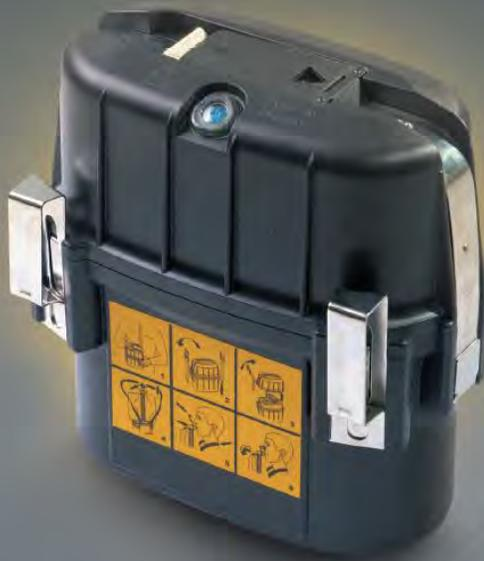
The Ci-30 KS is personal self-contained self-rescuer which uses chemical oxygen ( $KO_2$ ) to produce oxygen ( $O_2$ ) and absorb carbon dioxide ( $CO_2$ ). The Ci-30 KS is intended for use for escape from irrespirable atmosphere in case of underground accidents: fires, explosions, sudden release of gas or coal dust.
